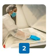
**Cover** area to be tested with wet absorbing side against the item. Sandwich the item to analyse both sides
