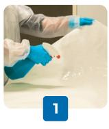
Cut a piece of STK Lab. Using a sprayer, **saturate STK Lab absorbing side** with demineralized water
